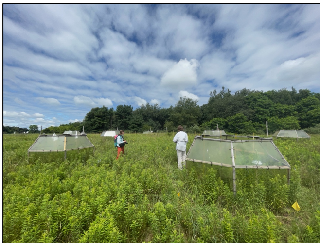
Open-topped chambers and control, ambient condition plots spread across a field at the Kellogg Biological Station.
