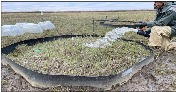
Top: Open-topped chambers increased the temperature over the experimental plots. Bottom: Researchers added brackish water to simulate flooding.
