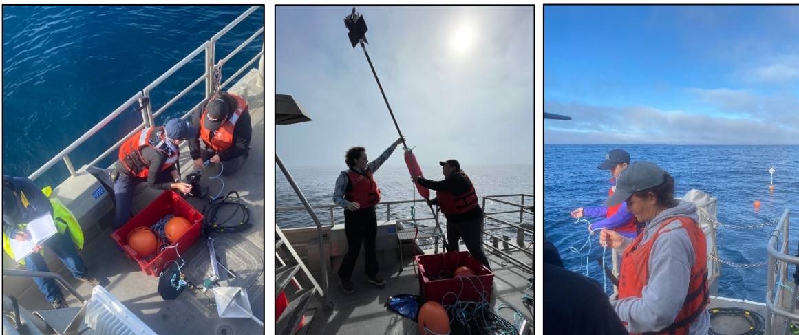
Deploying the drifting acoustic recorders: Scientists attach a weight to the line and wait to get into position (left), orient the pole buoy with the satellite transmitter on top (middle photo), and let out the line with the acoustic recorder and surface floats (right).
