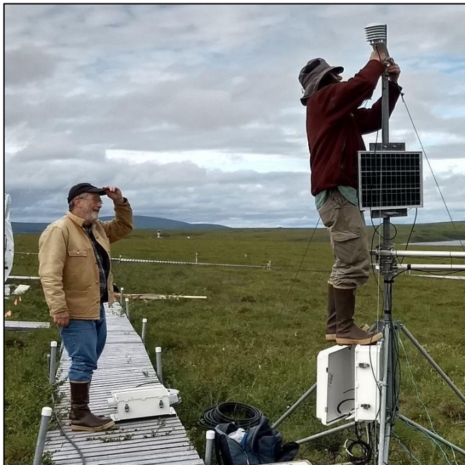
Gus (left) and Jim (right) set up a weather station to monitor air temperature and humidity on the tundra.
