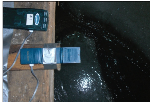
The sensor with data recorder on the dock inside a boathouse.
