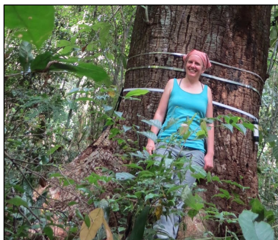
Kristina placed this band around a tree in Panama. It is used to measure growth.
