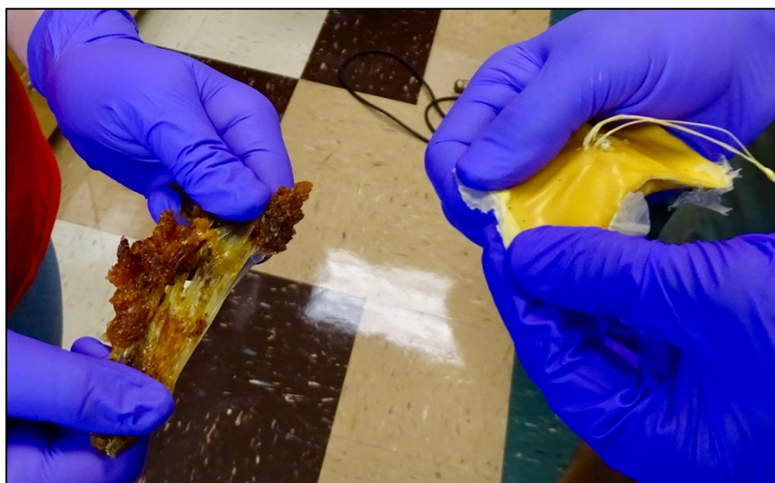
The sample on the right is made from 100% diglycerol and the left from 100% meso-erythritol.
