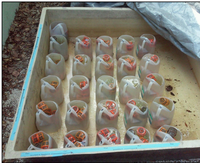
The experimental setup. Each container has a different concentration of phosphorus and salt.
