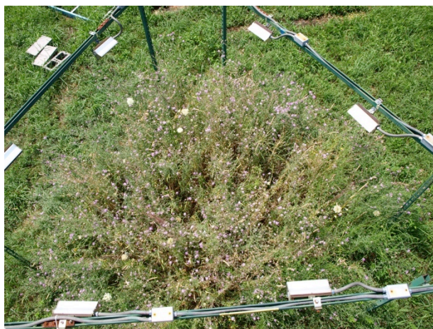
An aerial view showing one of the heated plots. The silver boxes are electric ceramic heaters, raising the temperature inside the ring.
