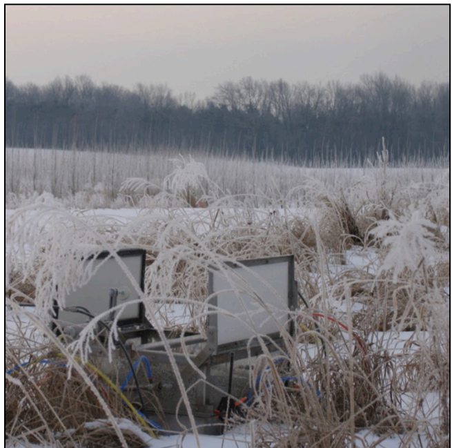
Measuring nitrogen ( N_2O ) gas escaping from the soil in a variety of conditions, like varying temperatures throughout the year. Photo credits: J.E. Doll MSU
